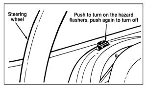
The control switch for the hazard flashers
